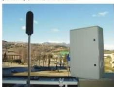
The choose of the monitoring system is the 1st step for right diagnostic. Sound level meters allows nowadays a huge amount of parameters recording, also for long time and with GSM - GPRS interface for remote control. It's very important to perform weather and traffic conditions monitoring to validate acoustic measurements and make useful correlation between records.
